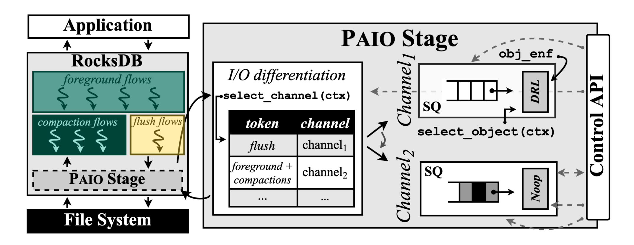
Identify the origin of POSIX operations (i.e., foreground, compaction, or flush operations)
