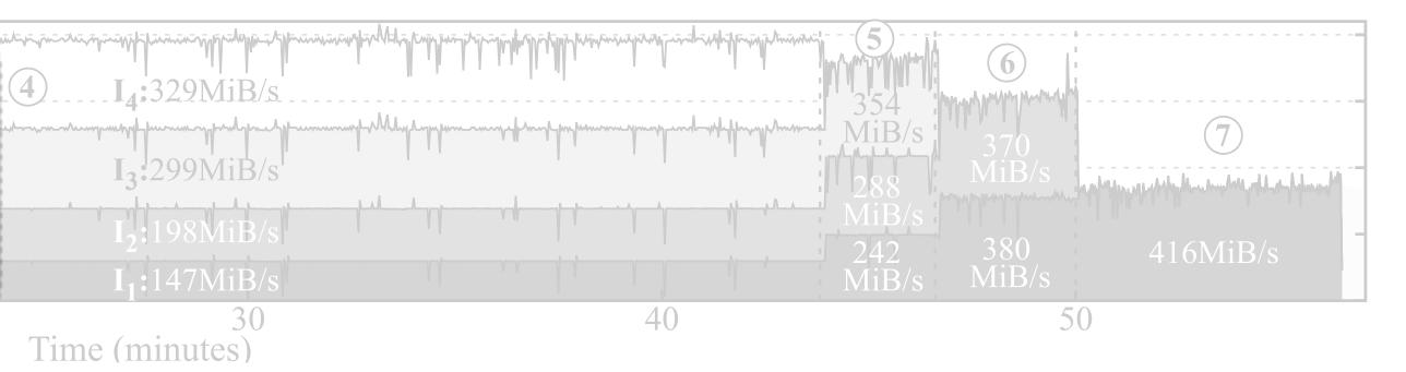
l<sub>3</sub> and l<sub>4</sub> cannot meet their bandwidth targets during 31 and 34 minutes
